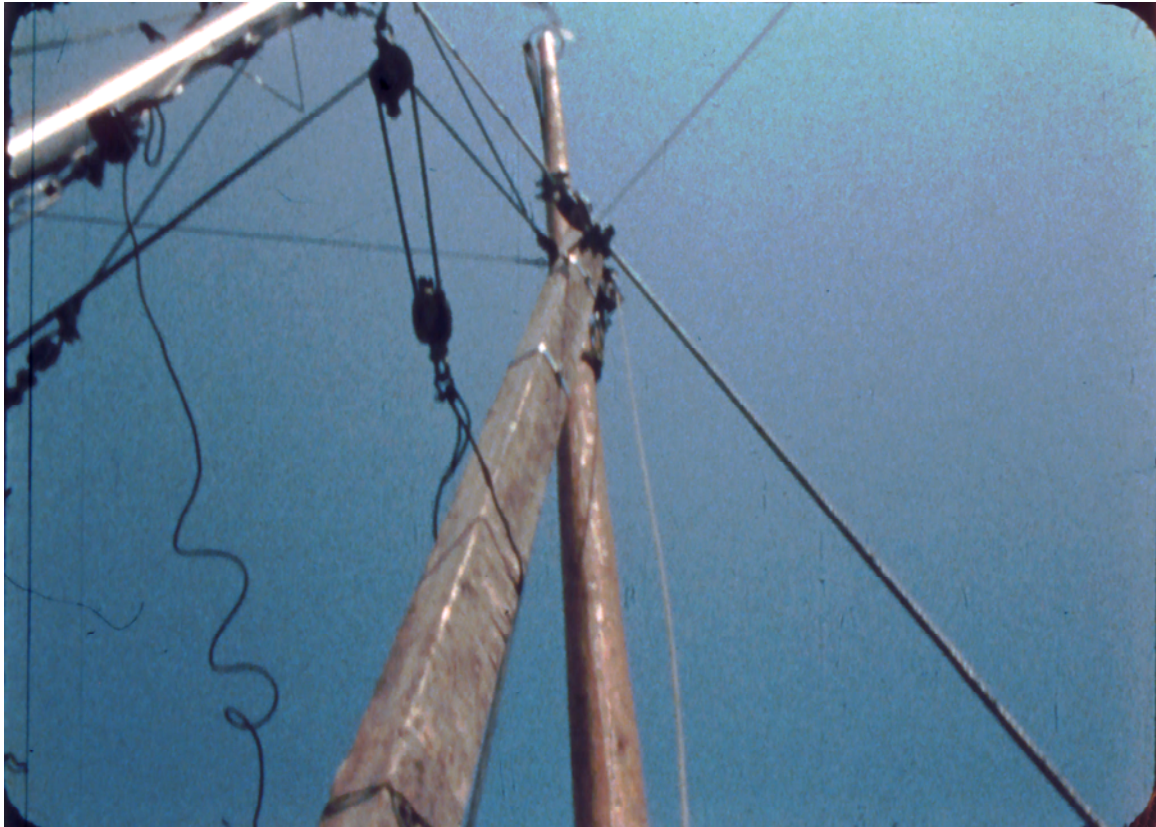
Hoisting the mast using a boom salvaged from the wreck of the "Rendezvous" near Mile Rock.
