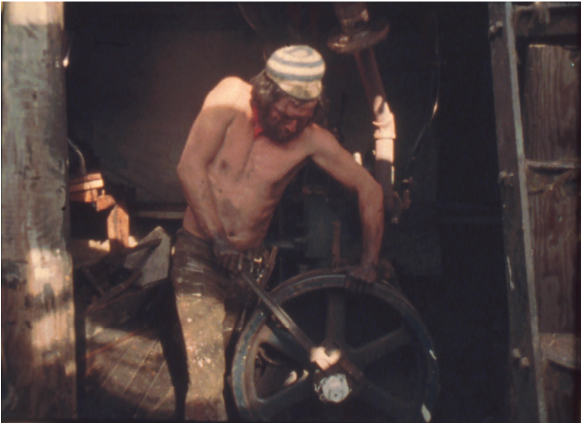
Installing the Hicks. This antique was made around 1906 and required hand starting.
